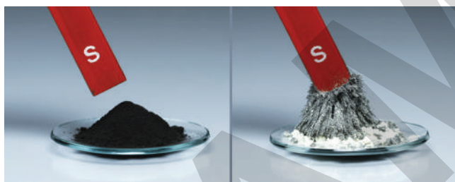
Figure 1.4: The iron in a mixture of iron and sulfur (left) retains its magnetic properties, but iron sulfide (right) is not magnetic.
