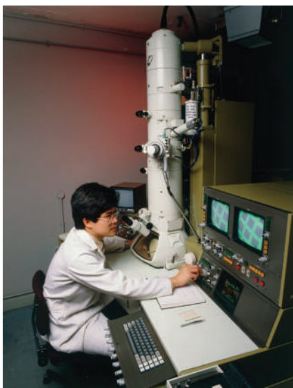
■ Figure A2.2.10 Using the transmission electron microscope
