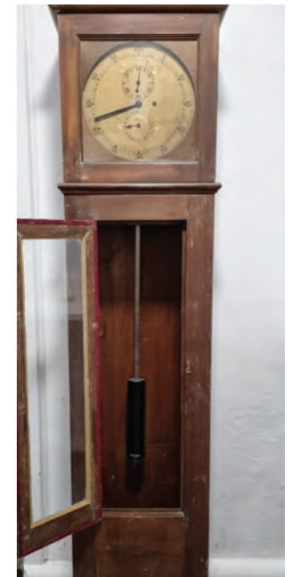
▲ Figure 1 Knowledge of simple harmonic motion led to the development of the pendulum clock. For about 300 years, pendulum clocks were the most precise clocks available. This is a sidereal clock used to help make astronomical observations.
